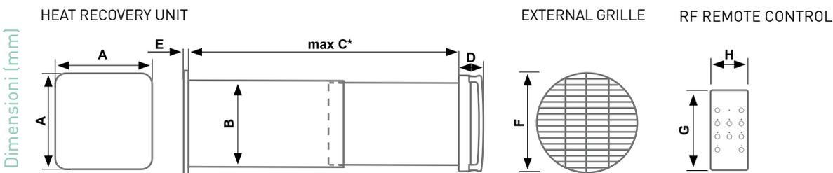
\* In case of wall thickness less than 280mm cut the telescopic tube to the needed length and use a standard external grille (not supplied with the product)
